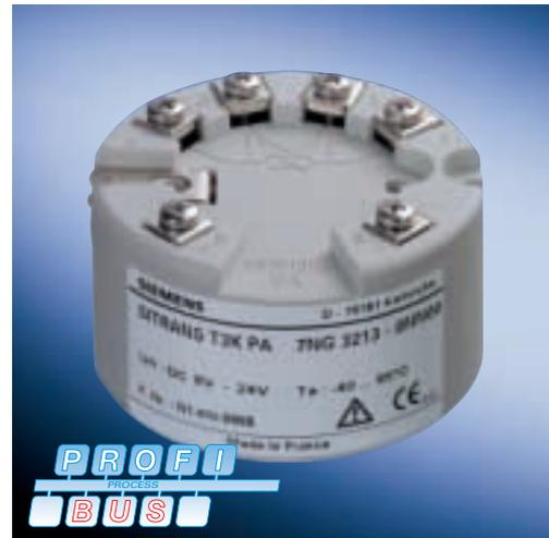
thermocouples and voltage sensors into digital signals. The measured value from the micro-processor is then placed on PROFIBUS PA. Sensor, limit values, failure mode, etc. are programmable. SITRANS T3K PA offers you a wide variety of diagnostic and simulation options.
